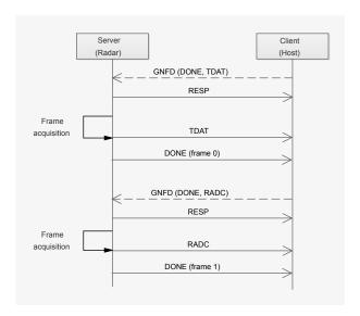
Figure 15: Read messages in streaming mode
