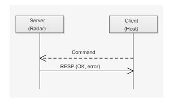
Every command sent by the client is acknowledged by the server with a response message (RESP). The response message includes an error code what delivers information data about the success or failure of the received command.
