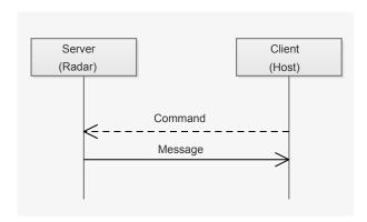
The communication is based on a client-server model. There are two types of packets transmitted. Commands are sent from client to server and messages are sent from server to client.
