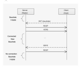
The server starts up with a default baud rate of 115200 baud. The client has to establish a connection with the INIT command where it needs to define the baud rate which will be used for the communication. After acknowledging of the INIT command by a RESP message a VERS message with a firmware string follows before the server changes the baud rate to the selected one out of the INIT command.
