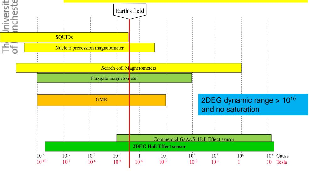
Fig.3. Magnetic field sensor spectrum
