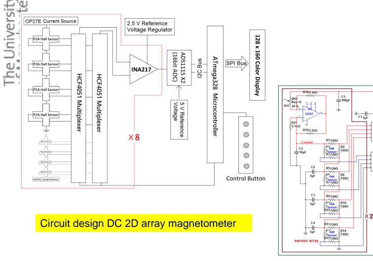
Schematic for DC 2D array magnetometer
