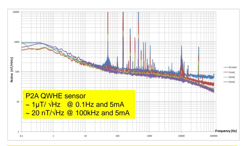
Fig. 6 Minimum B-Field detection as a function of frequency
