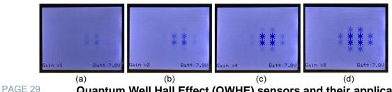
Sensitivity test results of the DC 2D Hall array magnetometer, where the attenuations in (a), (b), (c), and (d) are 1/32, 1/16, 1/8, and 1/4, respectively
