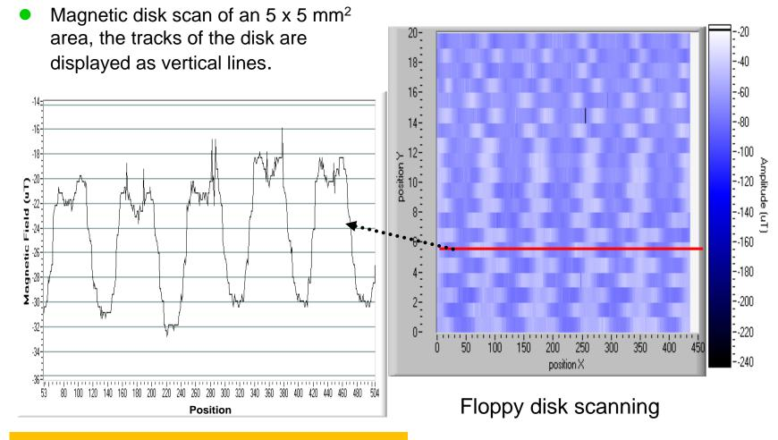
Figure 8. Cross section of red line , magnetic flux density variations ~ 10  $\mu T$
