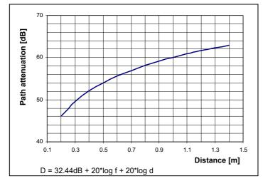
Fig. 12: Power attenuation over distance @24GHz
