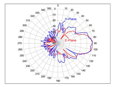
Fig. 3: Field Pattern of Tx Antenna
