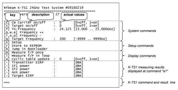
Fig. 4: K-TS1 output structure at a standard terminal program
