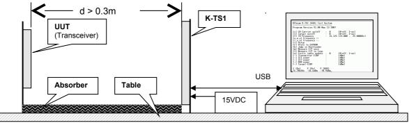
Fig. 11: Typical arrangement of a test-stand
