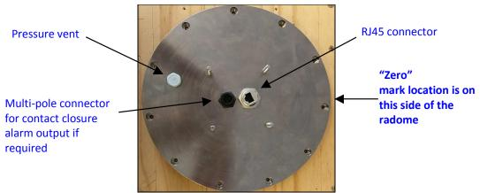
Radar base with 4 M6 fixing studs and "Zero" mark location
