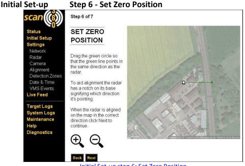
Initial Set-up step 6: Set Zero Position
