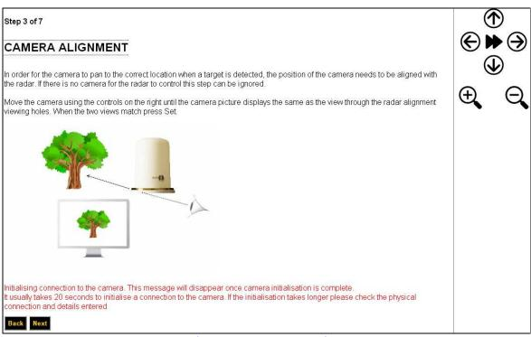
Initial Set-up step 3: Camera Alignment
