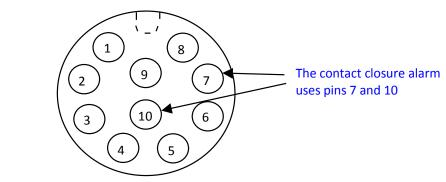
Solder-bucket end view of multi-pole cable connector pin-out (not supplied)
